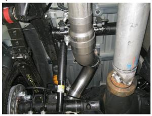
**Step 2.** Begin installation of the Magnaflow system by first clamping the 4"-5" Adapter Nipple to the newly cut outlet of the DPF using a supplied 4.00" clamp. Then attached the Over Axel Assy to the Adapter Nipple using the supplied 5" clamp and fitting the hangers in the rubber insulators (leave all clamps loose for final adjustment of the complete system).
