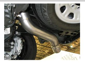
**Step 3.** Next Install the Tail Pipe Assembly in a similar fashion using the supplied 5.00" clamps and by fitting the welded hangers into the rubber insulators.
