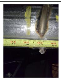
**Step 1.** To begin the removal of the OEM system you will need to cut 18.25" behind the DPF. You can then disengage the welded hangers from the rubber insulators, working rearward finish removing the system. Do not damage or discard the rubber insulators, as they will be reused to mount the new system.
