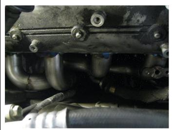
**Step 5.** Install your new header assemblies with the supplied gasket and header bolts to the manufacturers torque specifications. Reinstall the AIR connection on the drivers side assembly and the EGR and AIR pipes on the passengers side header assembly using the supplied gaskets.
