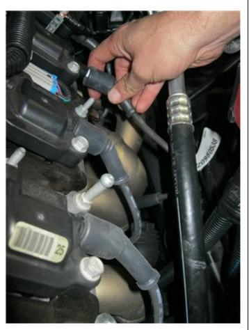
**Step 7.** Reinstall the spark plug wires to the ignition coils and the spark plugs. You will need to use the supplied 45deg spark plug wire to replace the OEM one located on the passengers side nearest the fire wall (Cylinder # 8). After all OEM parts have been reinstalled the battery can be reconnected.
