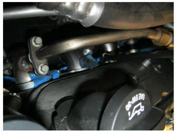
**Step 6.** Reinstall the OEM passenger side catalytic converters to the new header. Then reinstall the y-pipe assembly. Tighten the bolts and clamps to the manufacturers torque specifications. Reinstall the dipstick assembly, O2 sensors,
