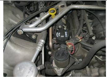
**Step 3.** Using a 16mm socket unbolt the dipstick assembly from the passenger side of the vehicle and remove.
