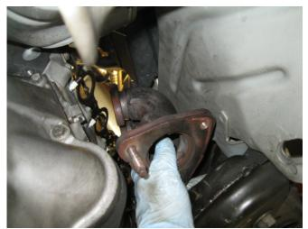
**Step 4.** At the top of each manifold unbolt both EGR pipes using a 10mm socket. Using a 10mm socket then unbolt both OEM manifold flanges. The OEM manifold assemblies can now be removed.
