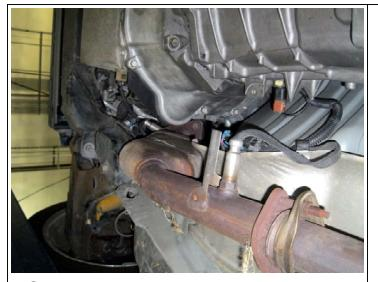
**Step 1.** Before removing the OEM header system, first disconnect the battery. Next remove all spark plug wires from the coils and the plugs, and then set aside. Using a 10mm socket unbolt the coil pack brackets from the driver side and passenger side and carefully flip them up towards the motor to keep out of the way. Using a 5/8" socket remove all of the spark plugs for clearance.
