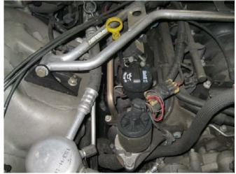
**Step 4.** Using a 16mm socket unbolt the dipstick assembly from the passenger side of the vehicle and remove.
