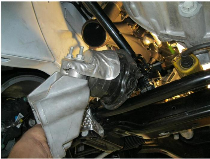
**Step 7.** Unbolt the driver side motor mount using a 15mm socket and then remove.
