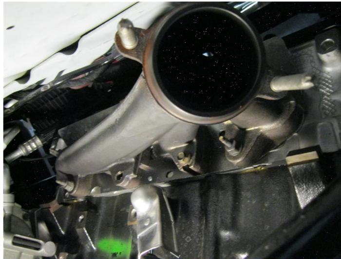
**Step 8.** After the motor mount has been removed unbolt and remove the OEM manifold using a 13mm socket. Using the gasket and bolts supplied install your new header using a 10mm socket to the manufacturers torque specifications. Then reinstall the driver side motor mount. Repeat the same process from removing the motor mount and OEM manifold to installing your new header assembly on the passenger side.
