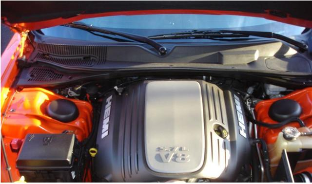
**Step 1.** Before removing the OEM header system, first disconnect the battery located in the vehicles trunk. Be sure not to close the trunk as it opens electronically. Disconnect air intake and set aside. Remove the engine cover by gently pulling to disengage it from the rubber grommets. Using a 10mm socket remove the engine coolant tank.
