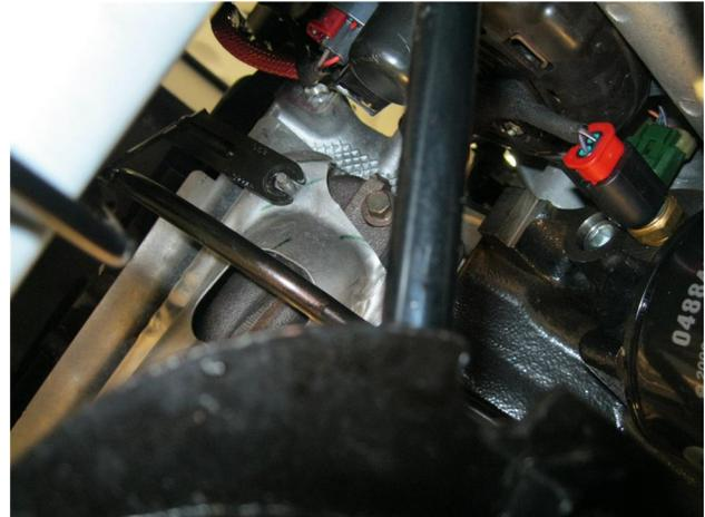
**Step 5.** Unbolt the dipstick assembly on the passenger side using a 10mm socket and remove.
