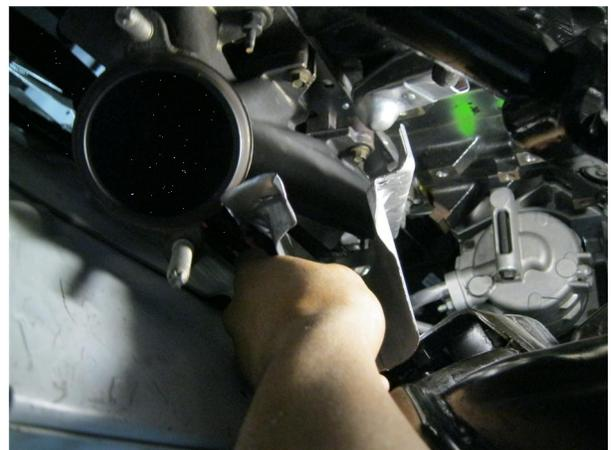
**Step 6.** Unbolt and remove the heat shields from both manifolds using a 10mm socket.
