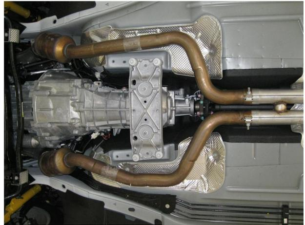
**Step 4.** Unbolt the driver side and passenger side catalytic converter assemblies from the manifold using a 10mm socket and remove. Unbolt the clamps on the back of both converter assemblies and then loosen. Both converter assemblies can now be removed.
