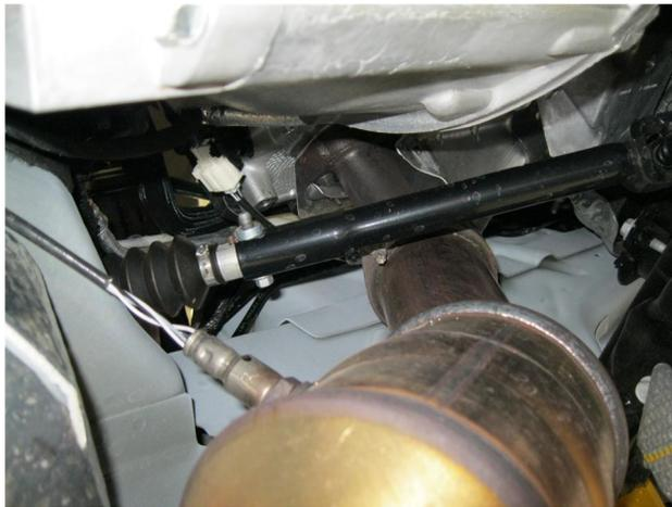
**Step 2.** Using a 7/8" wrench remove the O2 sensors located on the manifold and catalytic converter assemblies.
