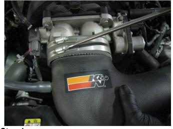
**Step 1.** Before removing the OEM manifold system, first disconnect the battery. Unbolt the air intake at the airbox inlet by loosening the retaining band clamp. This will allow you to rotate the engine for easier access.
