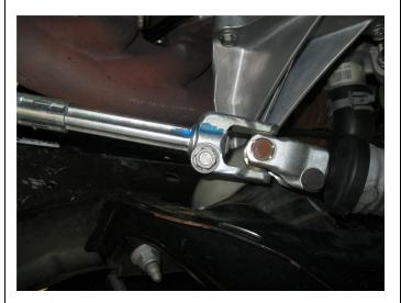
**Step 5.** Unplug the O2 sensor coupling for the header. When disengaging the steering shaft first mark both the shaft and the universal joint to ensure alignment on reassembly. Remove the retaining bolt and uncouple the steering shaft.
